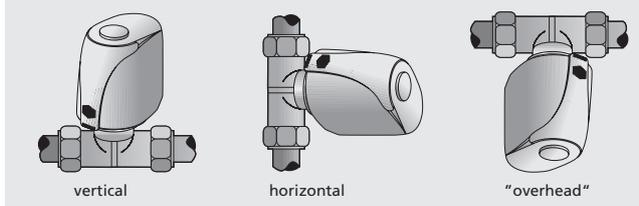
Preferred installation positions of the Alpha-Actuator are vertical and horizontal. An "overhead" position may reduce product life through special circumstances (e.g. contaminated water).
