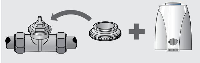
Valve adaptation is by means of a valve adapter which is available in different versions to suit to the most common valve bottoms and heating circuit distributors (please consider when ordering).
